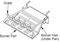
Figure 1 - Product Identification (Ramp Pan Burner)
